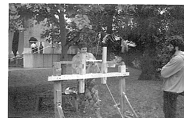
A Lathe or Wood Turner of Ancient Times. Notice the use of the branch as a spring.
